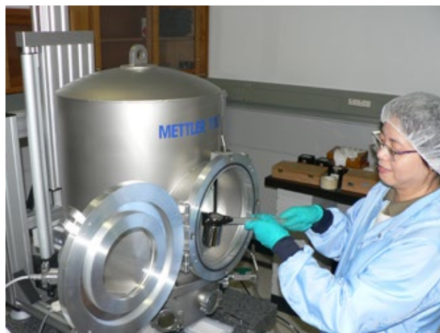
NMI scientist Kitty Fen comparing a stainless steel E0-level 1 kg mass with one of Australia’s two Pt-Ir kg references at the microgram level, in a pressure controlled chamber at the NMI.
