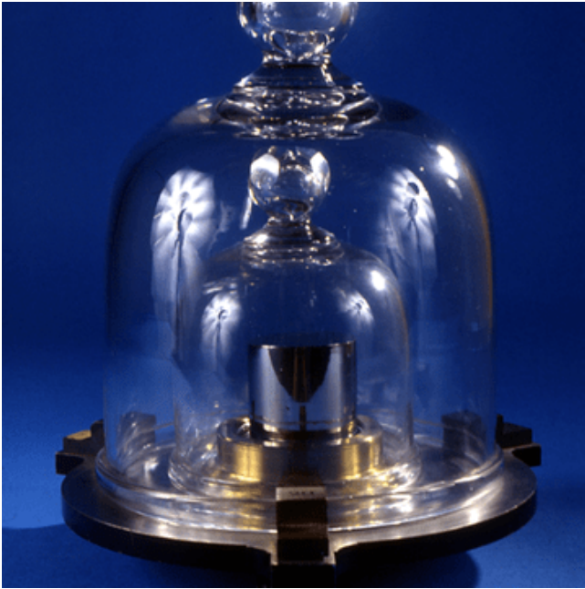
“Big K”, a Pt-Ir cylinder 39 mm in diameter and height, kept in a safe in the Pavillon de Breteuil near Paris — and defining mass throughout the universe!
