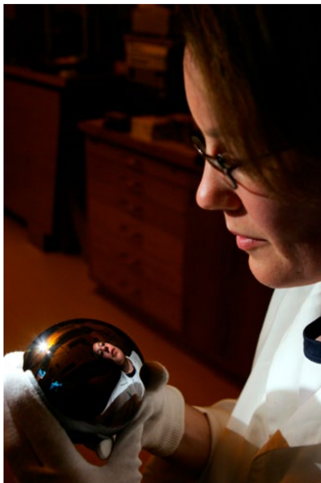
CSIRO scientist Katie Green inspecting a silicon sphere used in experiments to measure the Planck constant by relating the macroscopic SI mass units to atomic masses (photo: CSIRO, 2007).
